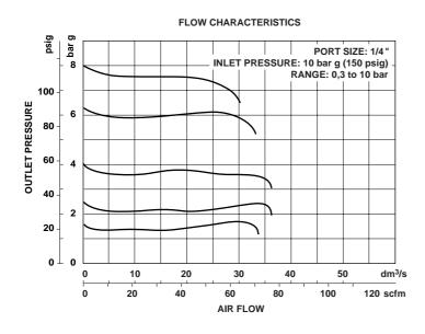
Ordering Information. Models listed include unidirectional flow, ISO G threads, knob adjustment, relieving diaphragm, 0,3 to 10 bar (5 to 150 psig) outlet pressure adjustment range\* without gauge.
